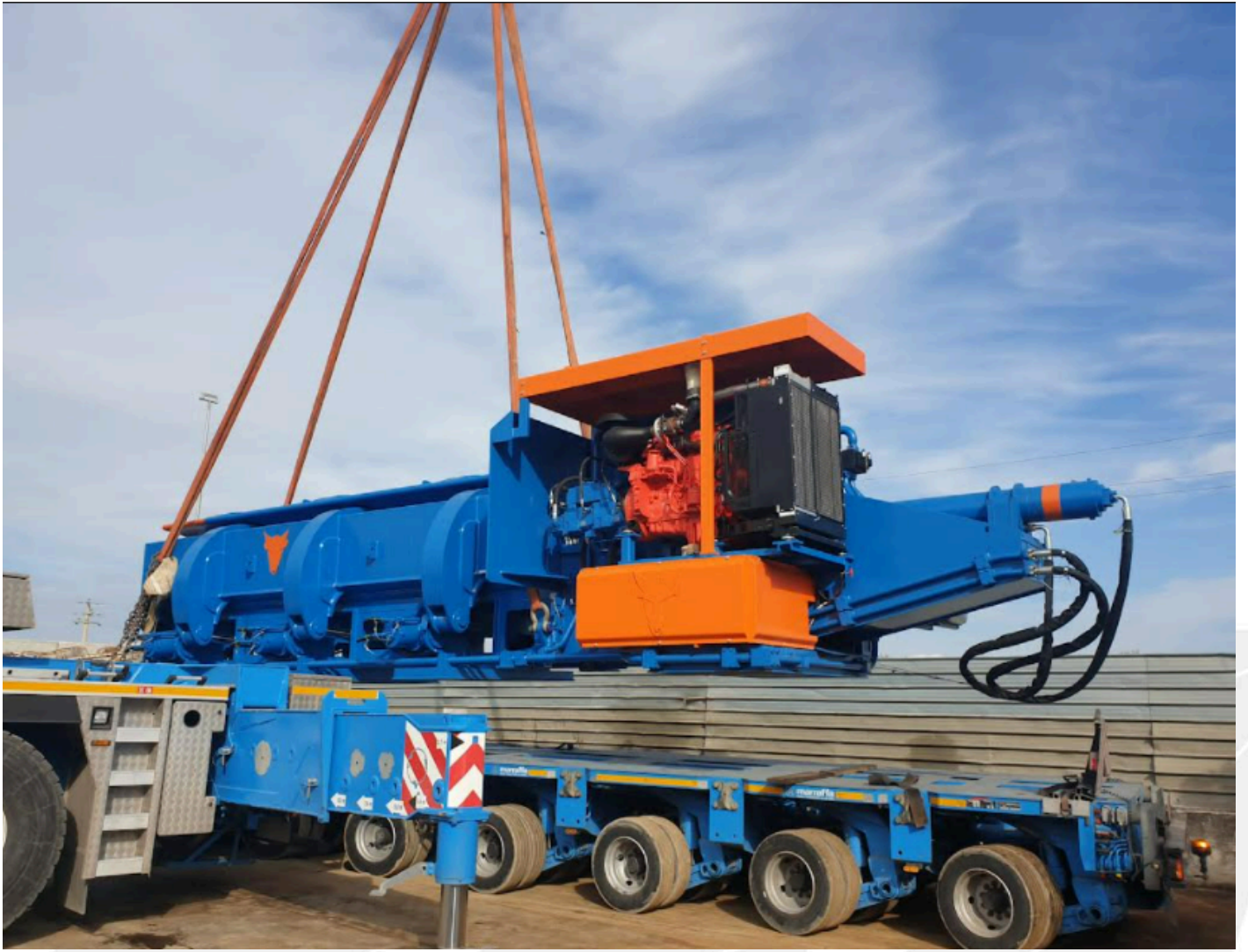
Shear Box shipped separate from Shear head (assembly by our staff)
