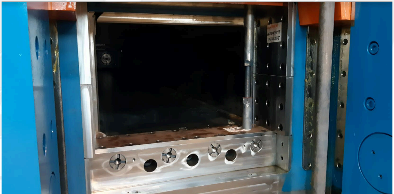
Shear Wear Plates and blade seats as discussed
