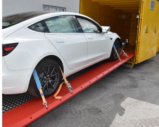
Rolling platform with chain driven operation
