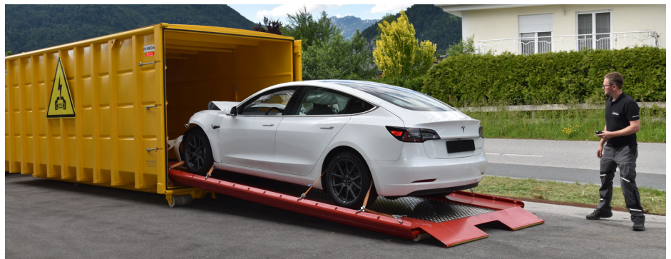
Operation of the retractable, chain driven rolling platform using remote control
