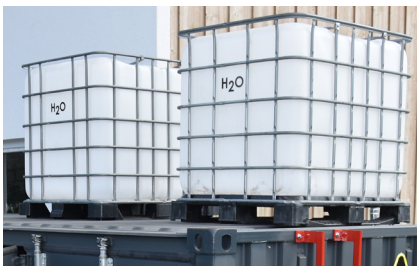
1000 lt water tanks mounted on the roof for flooding
