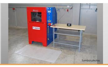
With the SEDA antistatic set, a potential equalization can be ensured simply and reliably, thereby preventing electrostatic charging in the hazardous area.
