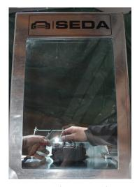
The connection to the airbag that needs to be neutralized happens behind a safe inspection window, which specifically protects the upper body area.
