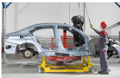
With the help of the load crane, e.g. the dashboard can be removed
