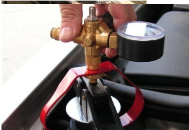
Pressure control valve
