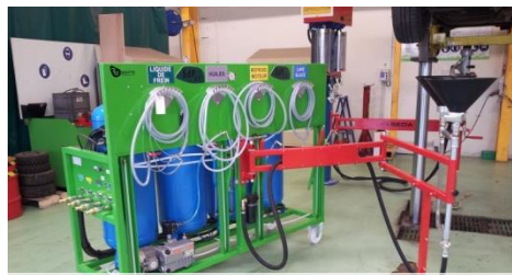
Full equipped de-pollution system
